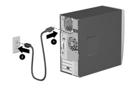
reconnecting the power cable on the \$0000/8000 (\$0000 shown)
